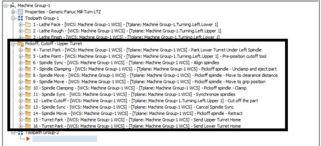
4. Edit Part-Off Op Just like in the POCO dialog input menu, each op's parameters can be adjusted. For example, if we want to change the feed rate of the part off tool, select op 12's Parameters and edit the Feed rate to 0.006. Click OK.
